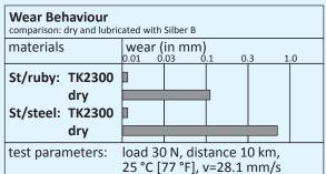
Lubrication of highly loaded, low or high-speed steel and jewel bearings up to pocket-watch calibers.
