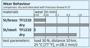
For metal/metal precision bearings (steel, non-ferrous
