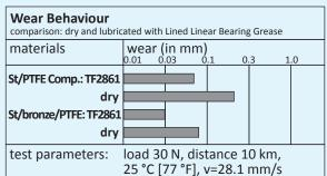
Special lubricant for highly loaded lined linear
